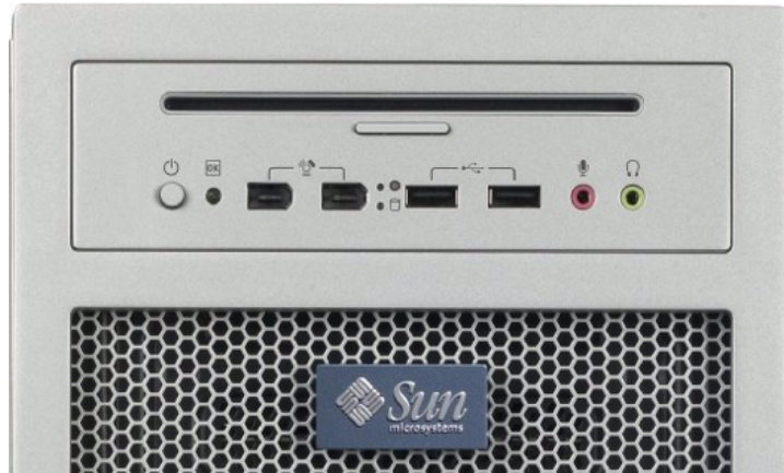
Figure 5. Sun Ultra 40 M2 workstation front perspective, featuring two FireWire ports, two USB 2.0 ports, microphone, and headphone jacks (left to right) in addition to a DVD-ROM/CD-RW or DVD-Dual (DVD+/-RW, dual layer capable) drive
